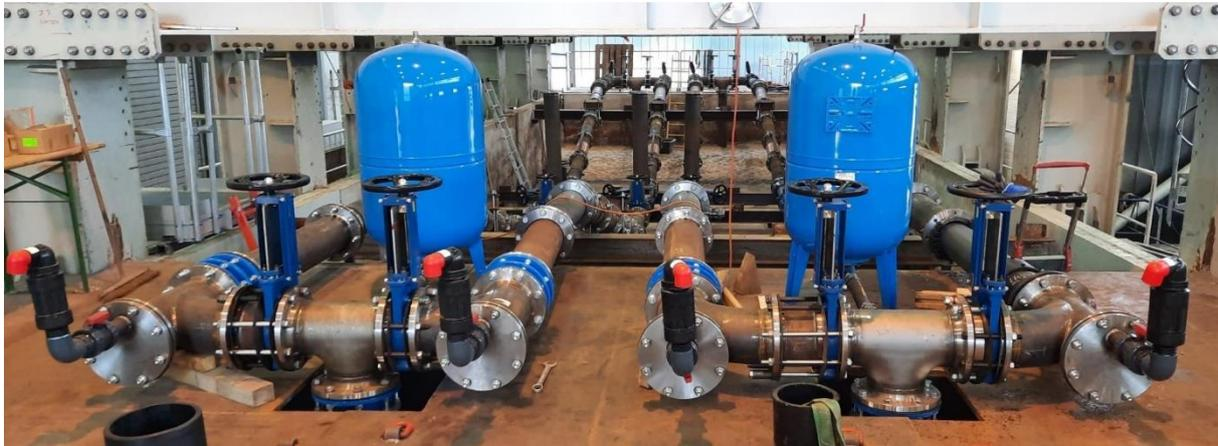
Figure 6. View of testing set-up in the IKT large-scale test facility from the front work platform showing the four installed pipes and blue pressure vessels.
