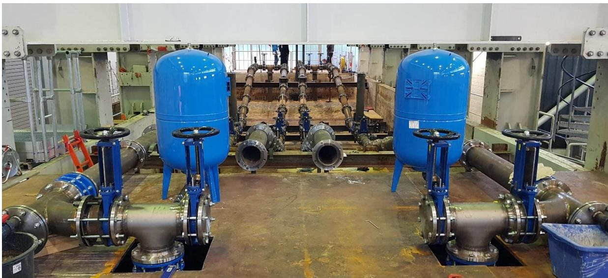
*Figure 9. Setup for initial evaluation of the hydraulic performance of undamaged steel pipe, before liner installation (test zero measurement). For pump 1 the continuous undamaged pipe run is on the left side of the test rig and pump 2 on the right side.*
