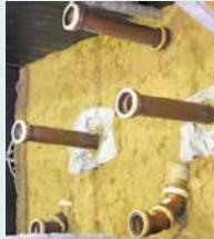
Rehabilitation task: Rehabilitation of three damage scenarios in each case in a non-rehabilitated vitrified-clay main sewer (DN 300)
