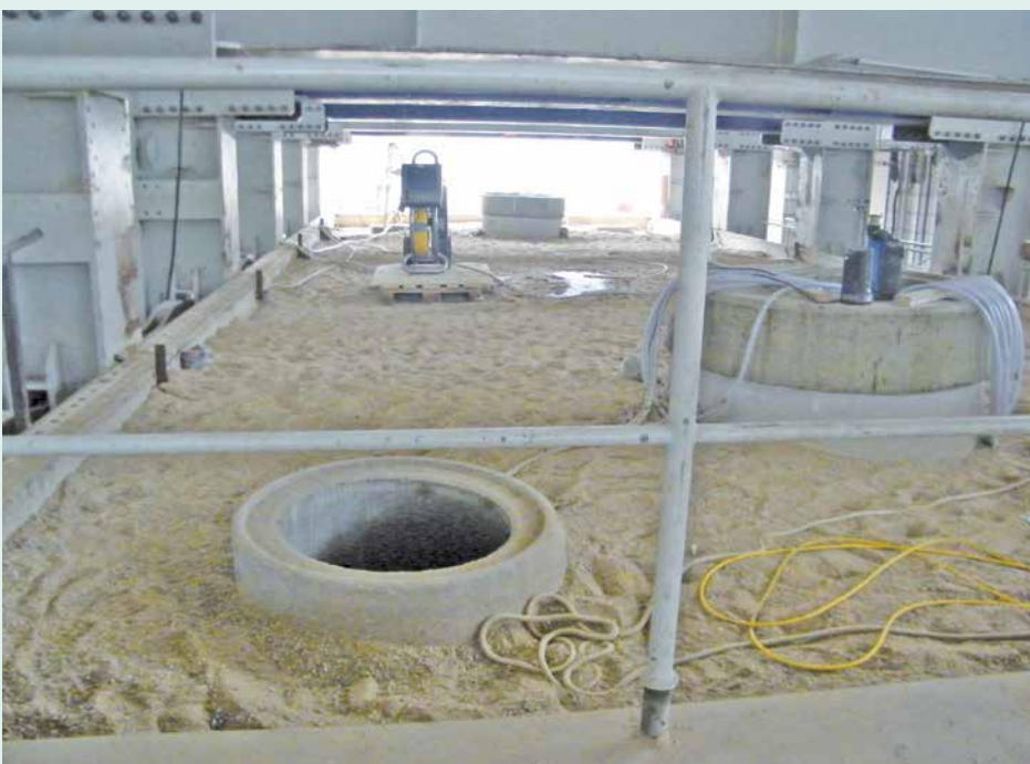
A giant sandpit: IKT's 6 m deep large-scale test facility can be flooded.
