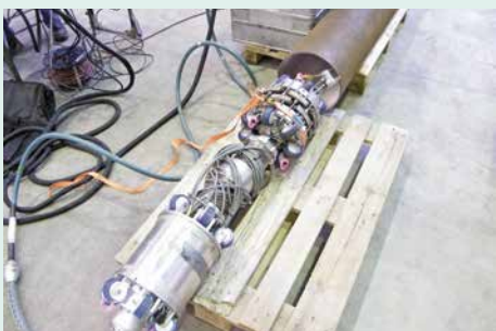
Eddy-current test (SloFec) in a pipe sample
