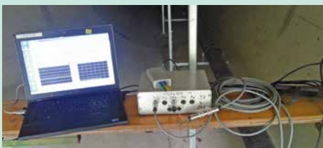
A laptop records pressure data during water-tightness testing
