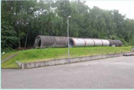
PE 100 test rig, installed in 30 m long concrete pipe DN 2200
