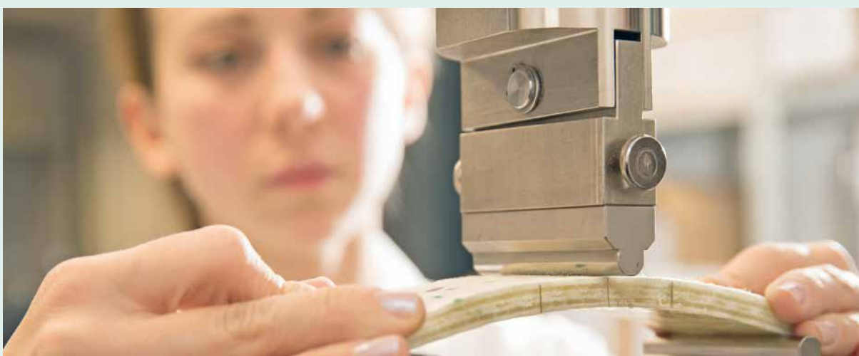
Three-point bending test on CIPP liners
