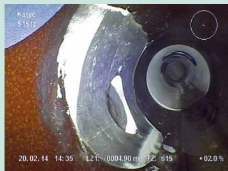
B: Tight lateral connection in vitrified-clay pipe
