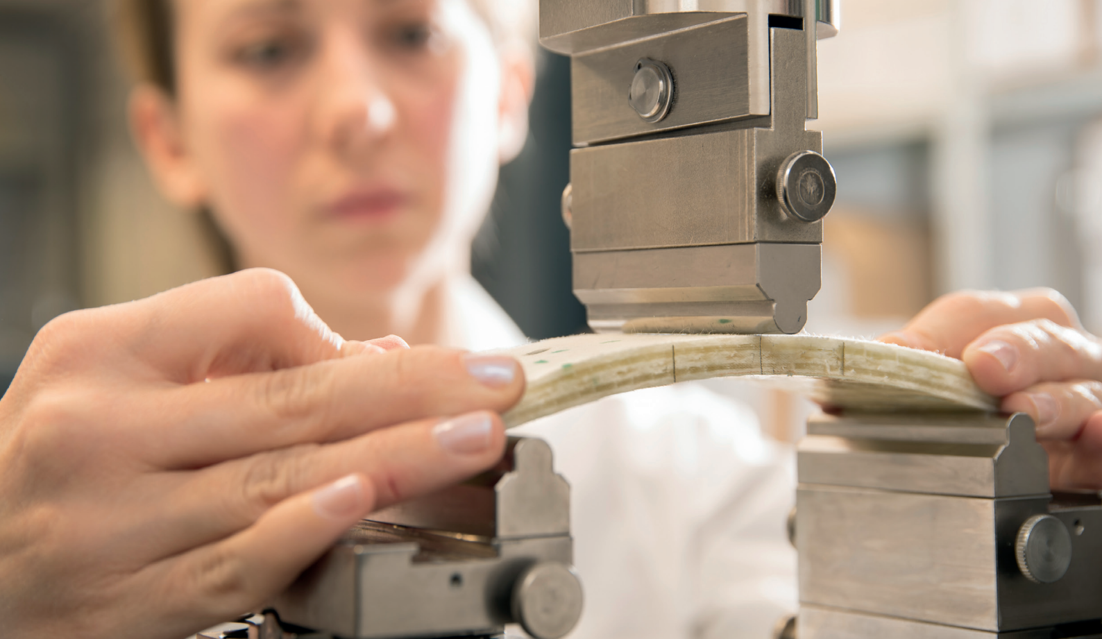
Three-point bending test on CIPP liners
