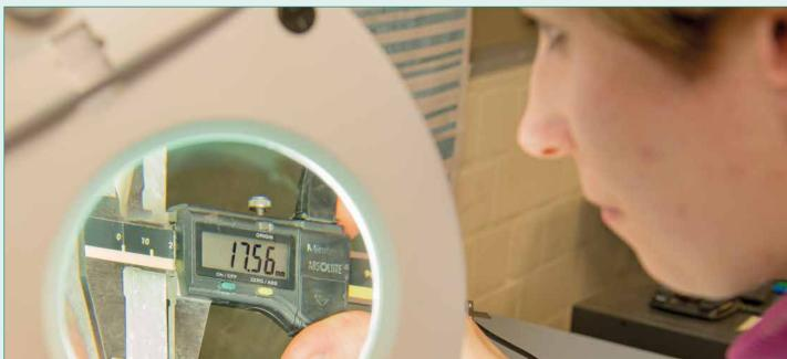
Precision slide gauge is used to measure combined thickness and the pure-resin layer
