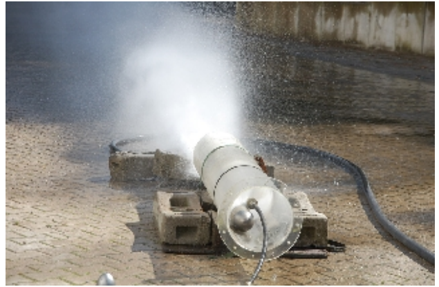
IKT Vehicle Check: determining pressure output at the nozzle
