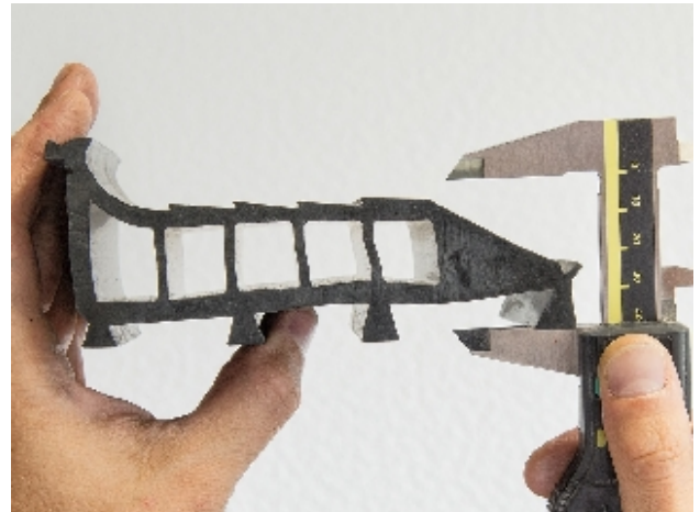
Testing of elastomers: Sealing width and contact pressure distribution
