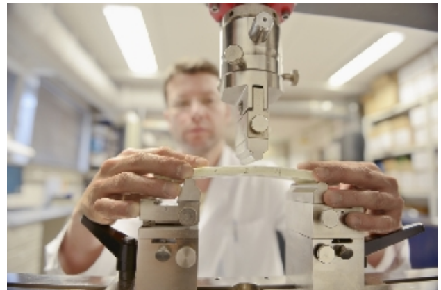
Three-point bending test on a CIPP-Liner
