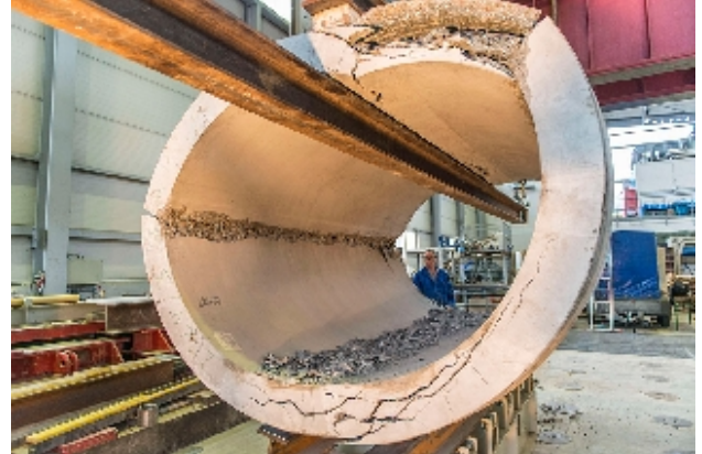
Vertical compression test on a reinforced-concrete pipe
