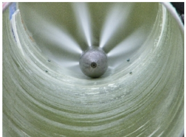
High-pressure jetting and flushing resistance (DIN 19523) – Practical test
