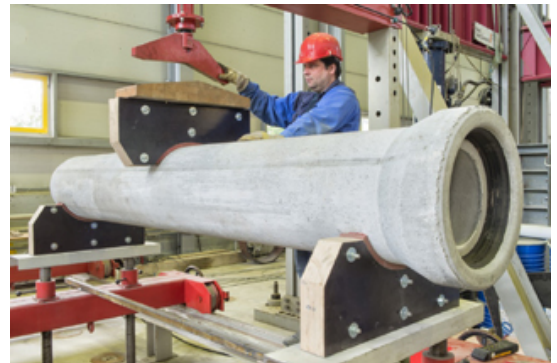
Determination of longitudinal flexural strength on DN300 pipes
