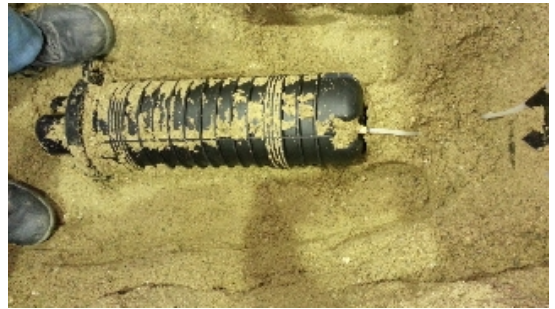
Tightness testing of buried fibre-optics splitters
