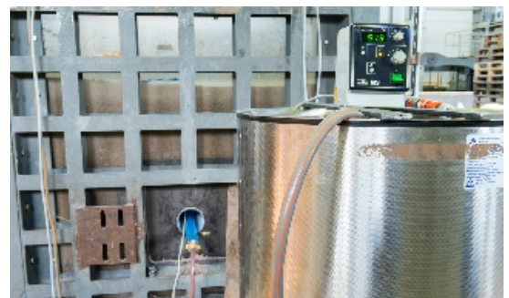
Measurement of temperature in buried sheathing pipes
