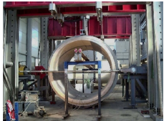
Modified vertical-compression test on large-calibre pipes
