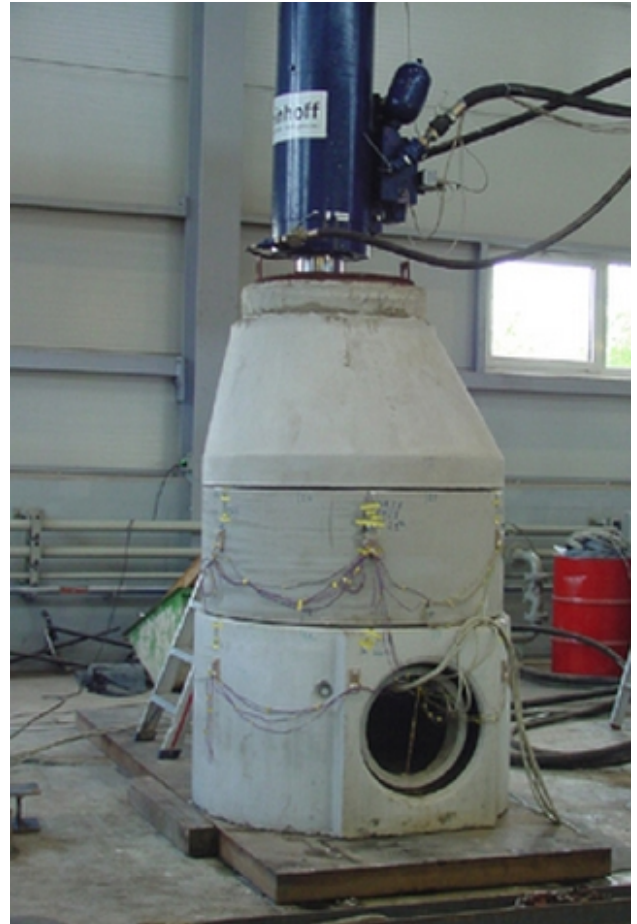
Deformation of manhole joints under vertical compressive load
