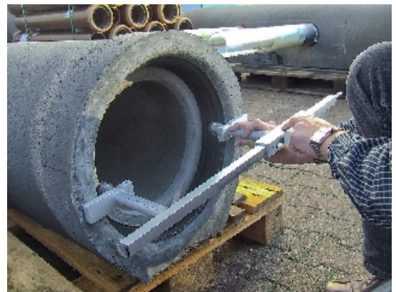
Measurement of concrete and reinforced-concrete pipes
