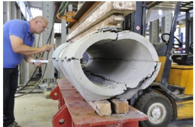
Vertical-compression test on a DN500 reinforced-concrete pipe
