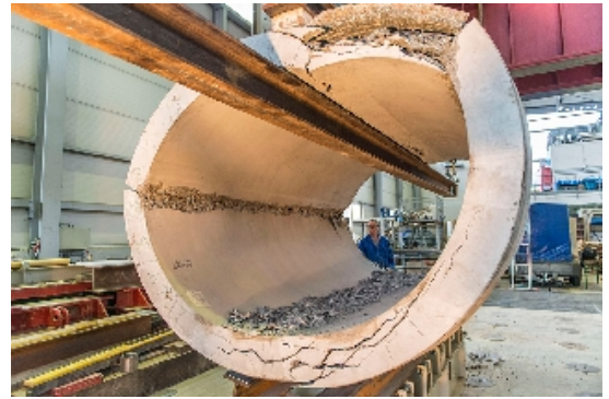
Vertical-compression tests on DN1600 jacking pipes
