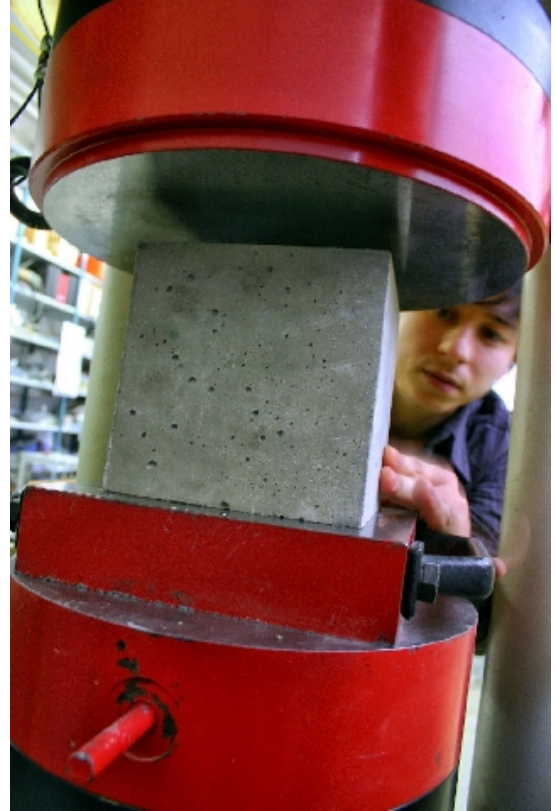
Testing strength in compression of concrete cubes
