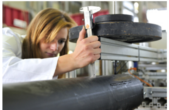
Determination of external abrasion on cast pipes
