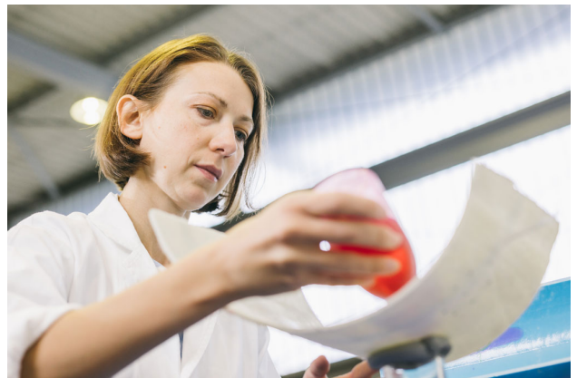
Water tightness test with red dyed water
