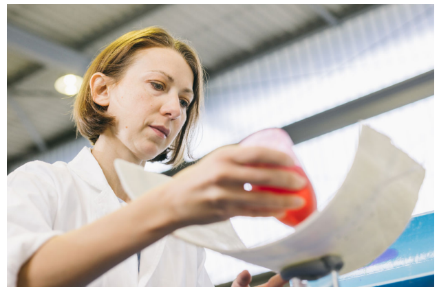
Water tightness test with red dyed water
