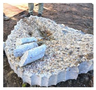
Extracted piece of host reinforced concrete pipe shows corrosion with coarse aggregates and dissolved reinforcement bars.
