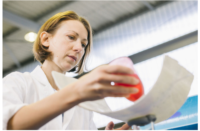
Water tightness test with red dyed water
