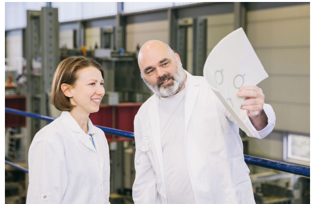
Initial assessment of a CIPP sample: searching for weak spots
