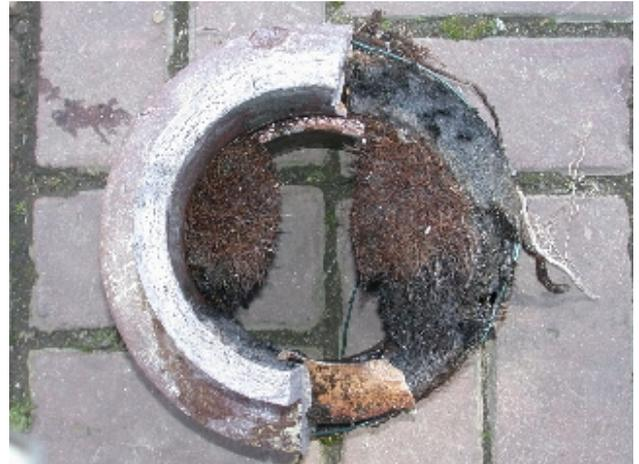
Pipe joint exhibiting severe root infiltration
