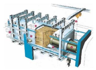
The IKT large-scale test facility: length 18 m, width 6 m, depth 6 m
