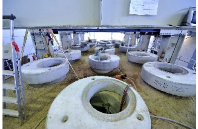
IKT's Comparative Test manhole renovation
