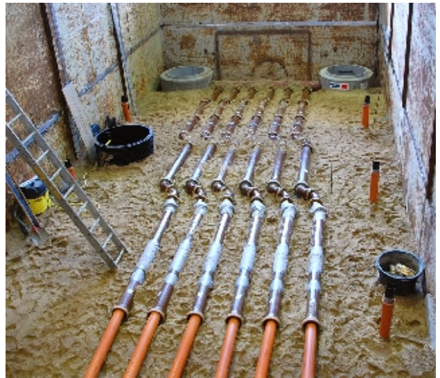
6 x 6 pipes: Layout of the test lengths in IKT's large-scale test facility
