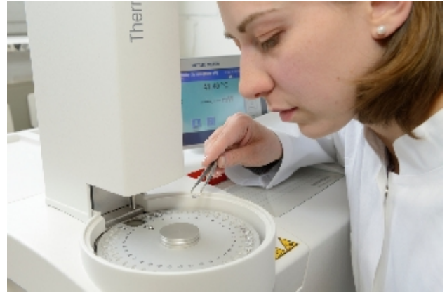
DSC analysis of resin samples
