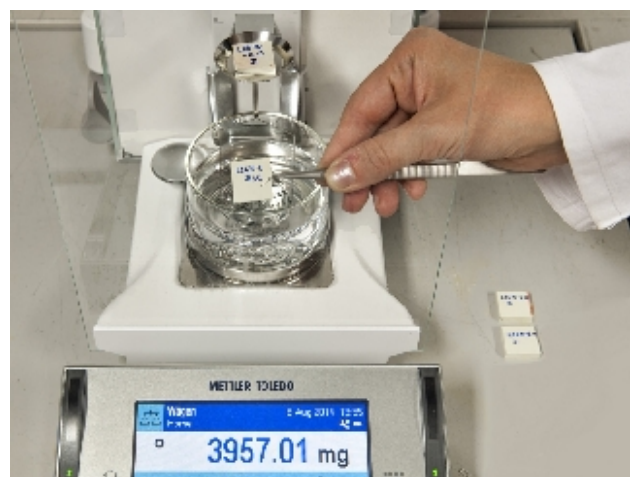
Precision scale for determination of density
