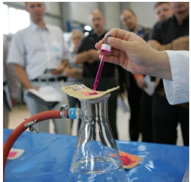
Water-tightness test on a CIPP-liner
