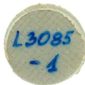
Sample for DSC analysis: 20 mm
