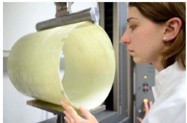
Major topic: CIPP and quality control – crown pressure test on a CIPP liner
