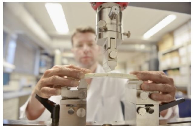
Three-point bending test on a CIPP-Liner
