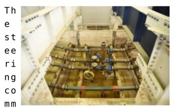
$_{\mbox{it}}\mbox{\sc View}$  of the built-in sewer pressure pipelines in the IKT telarge 1:1 scale test facility
