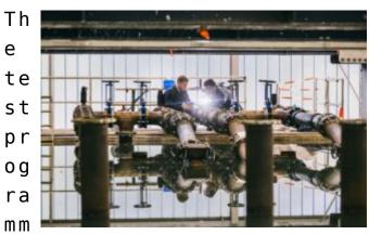
$_{\rm e}$  Simulation of external water pressure: After flooding, part  $_{\rm c\,o}$  of the test setup is reflected in the water
