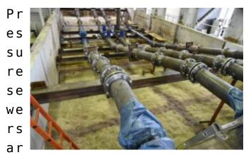
e Experimental setup of pressure sewer pipes in the IKT large
