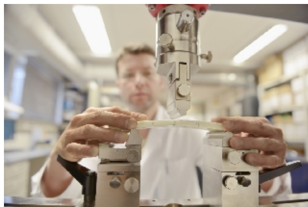
Three-point bending test on a CIPP-Liner
