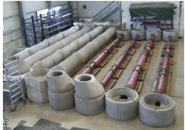
Test apparatus for short-liners and internal sleeves
