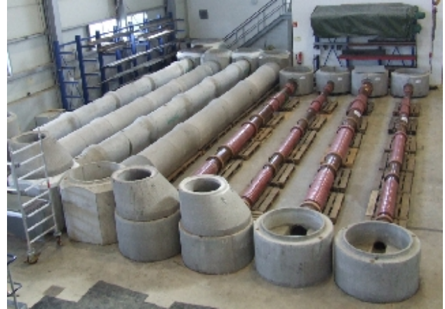
Test apparatus for short-liners and internal sleeves
