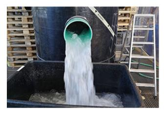
What comes out the other side? The NJDEP test procedure determines the retention capacity of the system.
