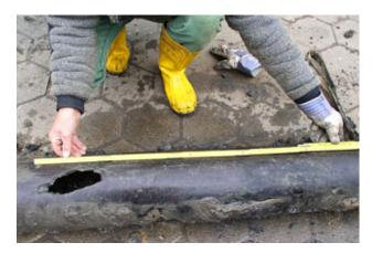
Investigation the applicability and limitations of the first rehabilitation techniques for pressure sewer pipes
