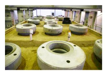
On-site installation conditions simulated in IKT's large-scale test facility — here with manholes to test and compare rehabilitation methods
