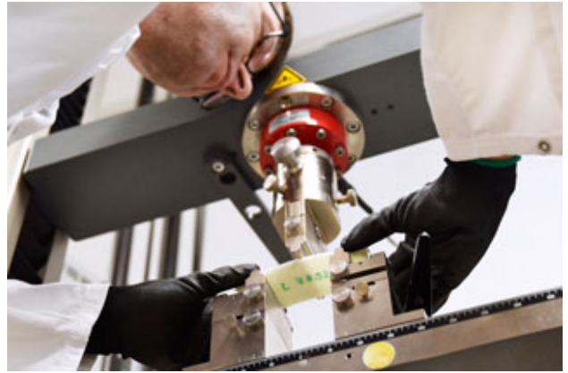
Three-point bending test: mechanical testing of modulus of elasticity and bending strength
