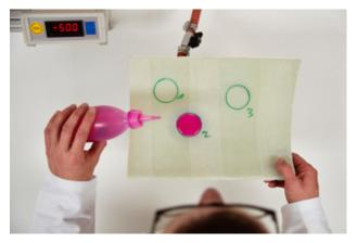
Under vacuum pressure: the test fluid leaked through the laminate in very few samples.
