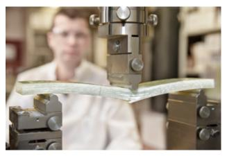
Under pressure: An IKT tester determines flexural strength at the point when a liner sample ruptures.
