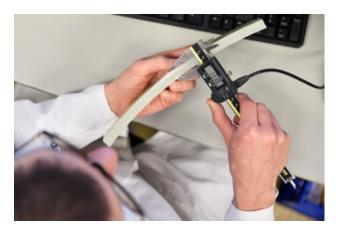
Wall thickness: wide distribution of results with lowest-scoring company passing only 60% of the tests
