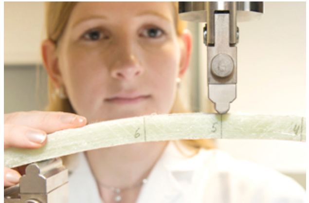
Three-point bending test on a CIPP liner
