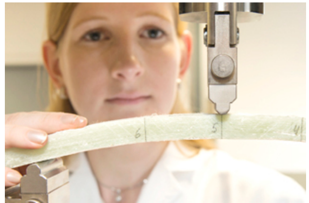
Three-point bending test on a CIPP liner
