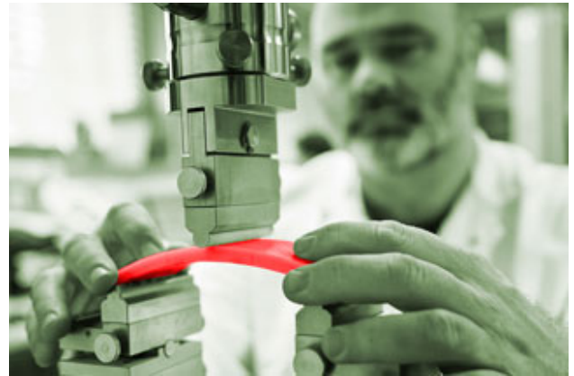
Three-point bending test: mechanical testing of modulus of elasticity and flexural strength
