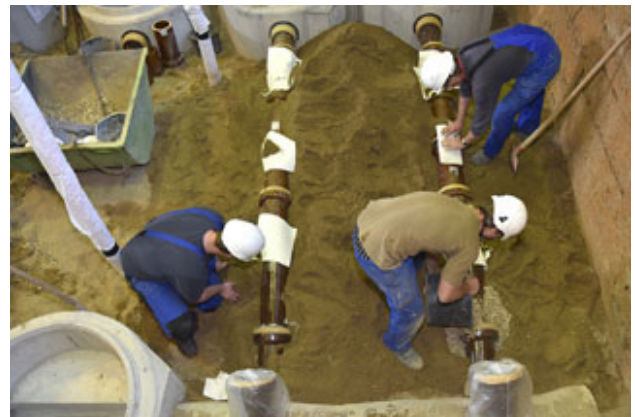
Defined damages: preparing the test rigs
