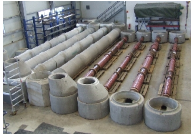
Test apparatus for short-liners and internal sleeves
