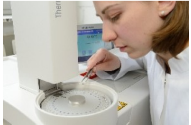
DSC analysis of resin samples
